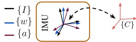
Fig. 1. IMU sensor composed of accelerometer and gyroscope. The base “inertial” frame  $\{I\}$  can be determined to coincide with either accelerometer frame  $\{a\}$  or gyroscope frame  $\{w\}$ .  $\{C\}$  represents the camera frame.
