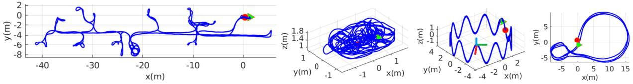
Fig. 2. Simulated trajectories. Left: *tum\_corridor* with fully excited 3-D motion; Middle left: *tum\_room* with 1 axis rotation and 3-D translation; Middle right: *sine\_3d* with constant centripetal acceleration along local IMU *x*-axis (red-axis). Right: *udel\_gore* planar motion with constant *z* and only yaw rotation. The green triangle and red circle denote the beginning and ending of these trajectories, respectively.
