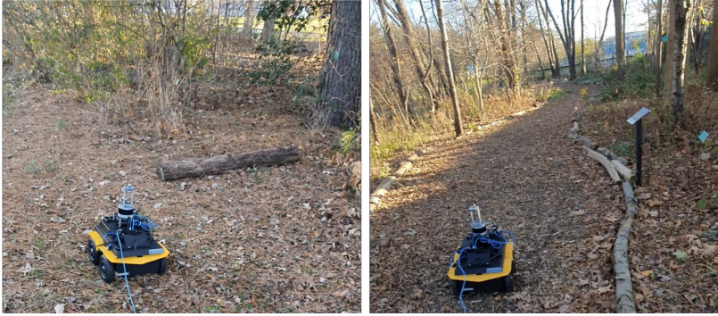
Fig. 1. A Clearpath Robotics Jackal robot moving autonomously along a trail within a wooded outdoor space. Under a thick canopy in such environments autonomous robots should be able to localize and navigate without relying on GPS. (The Ethernet cable visible was utilized solely for remote data collection and telemetry.)
