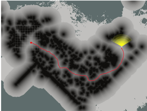
Fig. 10. The final Jackal position and costmap generated in the outdoor wooded environment. Black regions represent obstacles (trees or fence structures).
