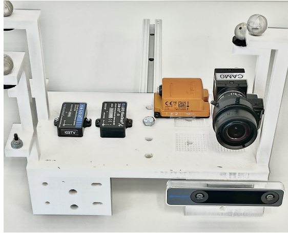
Figure 14: Visual-Inertial Sensor Rig contains a MicroStrain GX5-25 IMU, MicroStrain GX5-35, Xsens MTi 100, FLIR Blackfly camera and RealSense T265 tracking camera. The RealSense T265 tracking camera contains an integrated IMU and a fisheye stereo camera.
