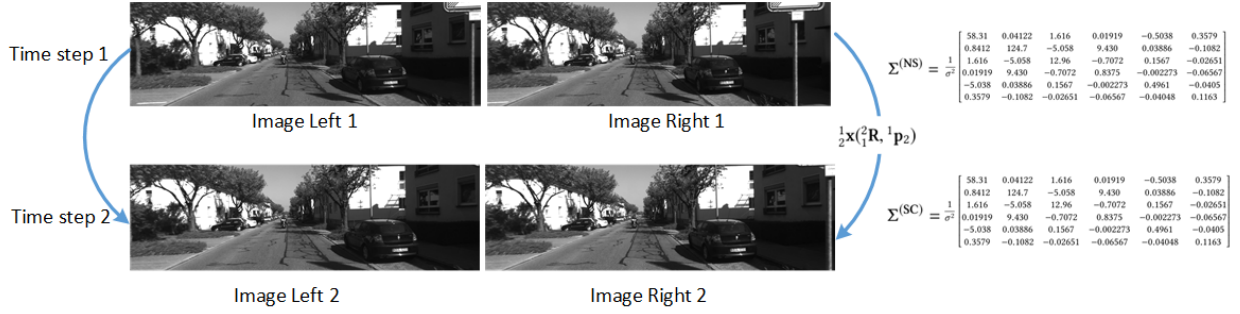
Fig. 2. A typical vision factor for visual odometry. \frac{1}{2}\mathbf{x}(\mathbf{R}_1, \mathbf{p}_2) represents the transformation from stereo camera pose 1 to pose 2, where \mathbf{R}_1 and \mathbf{p}_2 denote the rotation and translation between pose 1 and pose 2, respectively.
